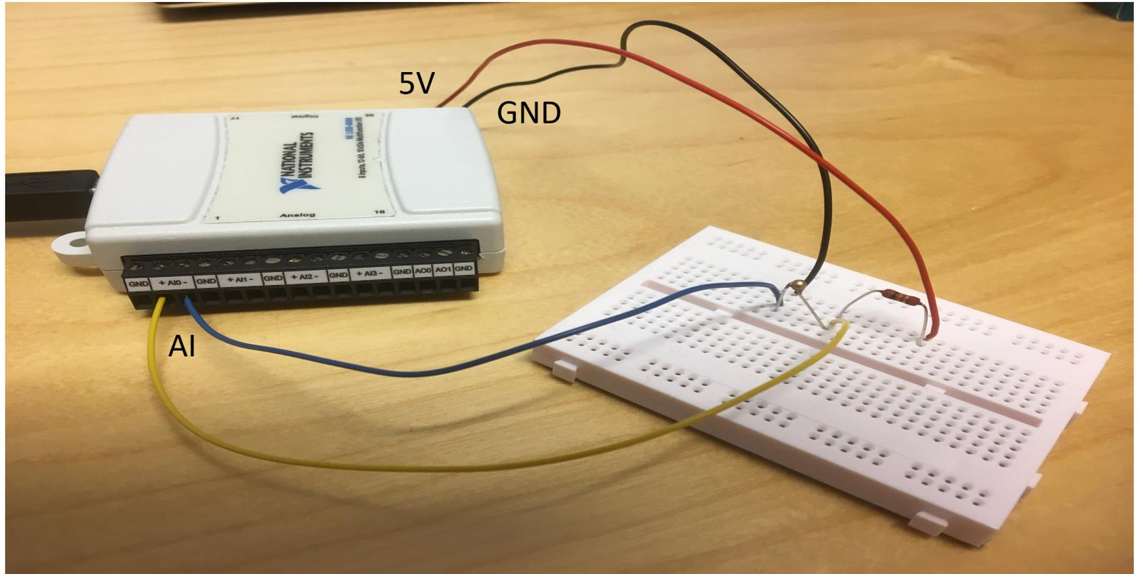
We connect the TMP36 to LabVIEW using a USB DAQ Device from National Instruments, e.g., USB-6001, USB-6008 or similar. I have used a breadboard for the wiring.
