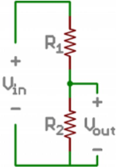
$$V_{out} = V_{in} \cdot \frac{R_2}{R_1 + R_2}$$
