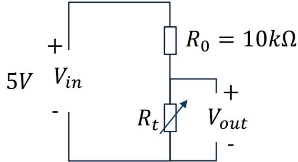
$R_t$  - 10k Thermistor. This varies with temperature. From Datasheet we know that  $R_t = 10k\Omega @ 25^\circ\text{C}$
