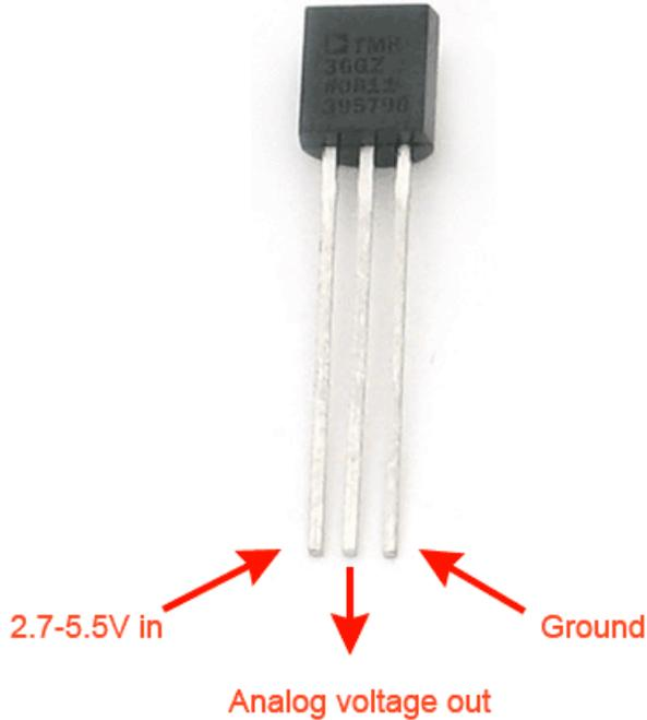
A Temperature sensor like TM36 use a solid-state technique to determine the temperature.
