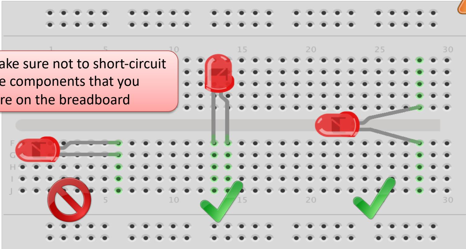
The Breadboard is used to connect components and electrical circuits
