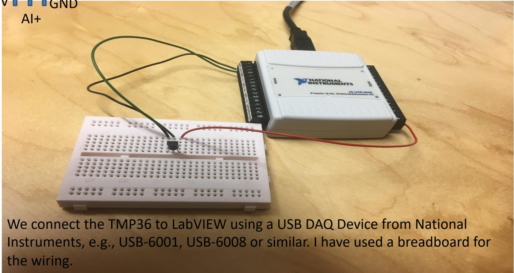
We connect the TMP36 to LabVIEW using a USB DAQ Device from National Instruments, e.g., USB-6001, USB-6008 or similar. I have used a breadboard for the wiring.
